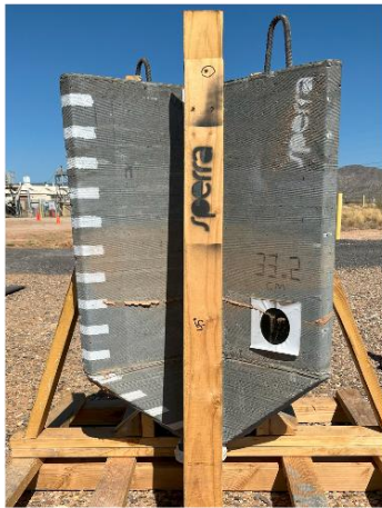
Concrete Anchors - 45° Angle
