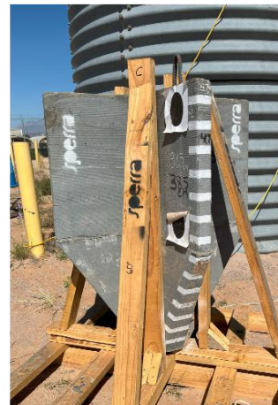
Concrete Anchors - 60° Angle
