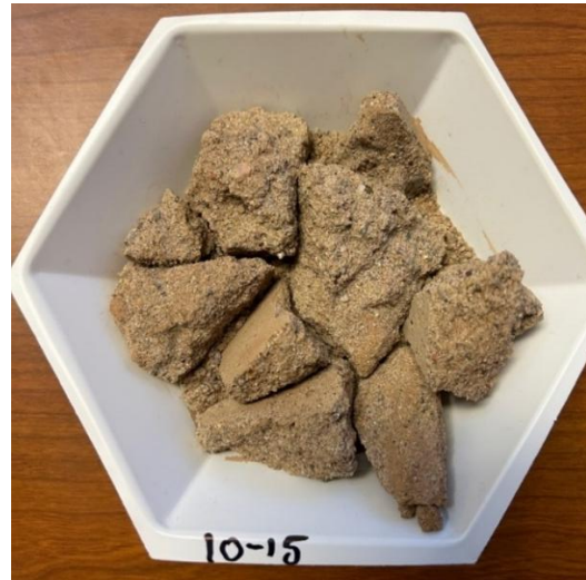
Figure 14. Picture of 10-15 cm depth sample after being dried in the oven.
