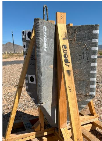
Concrete Anchors - 52.5° Angle
