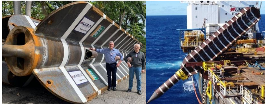
Figure 1. 100-ton steel torpedo anchor for the oil and gas industry. Smaller units will be appropriate for marine energy's lower loads.
